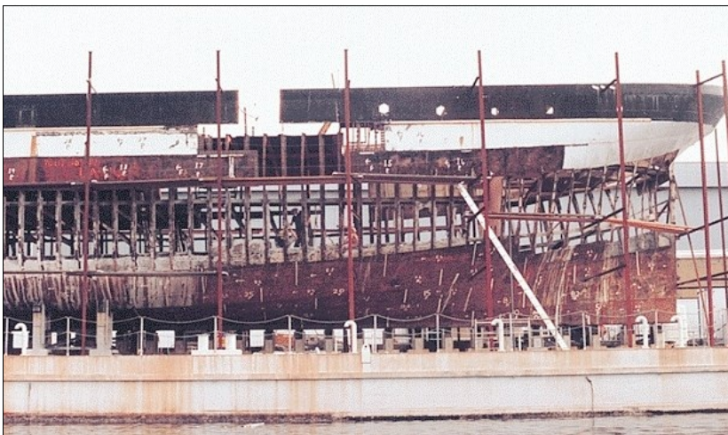
The stern of “JamesCraig” with plates along the waterline removed. She is on her pontoon in the Sea Heritage Dock in Sydney. No date, but likely the early 1990s. Image: SHF.
