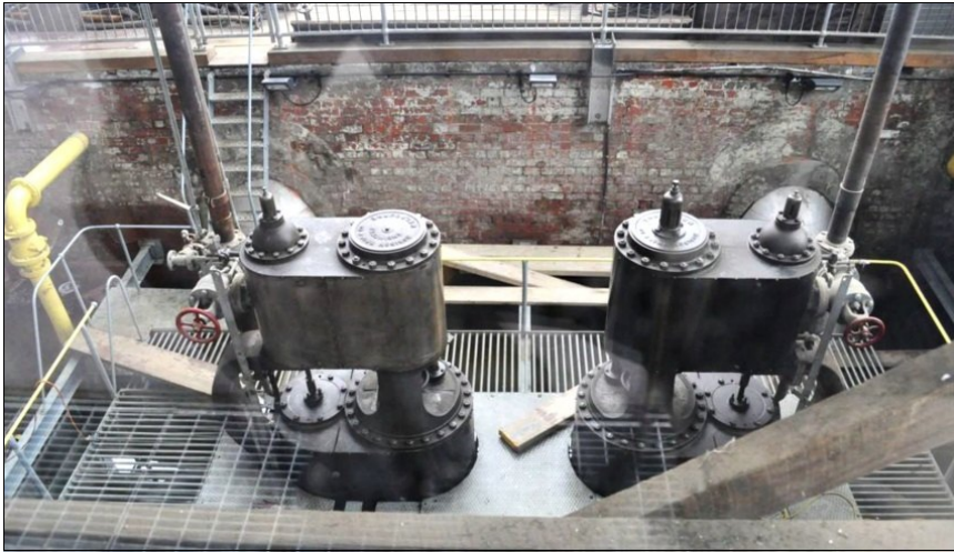
High pressure cylinders of the Duke & Orr pumping engine, with the top of the low pressure cylinders below them, and just projecting above the operating platform. Photographed through the glass wall, hence the shadowy reflections of metal grilles. Image: Owen Peake.
