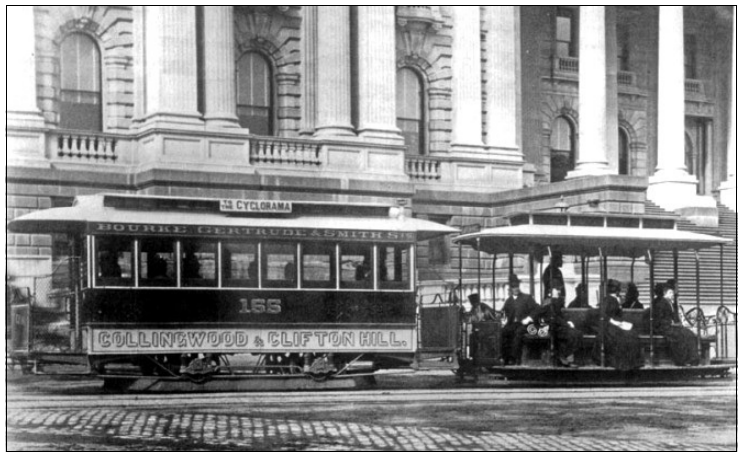
A cable tram on Spring St, Melbourne, in front of Parliament House. The motive car with cable grips is at right, closed trailer car at left. Image: "Walking Melbourne".
