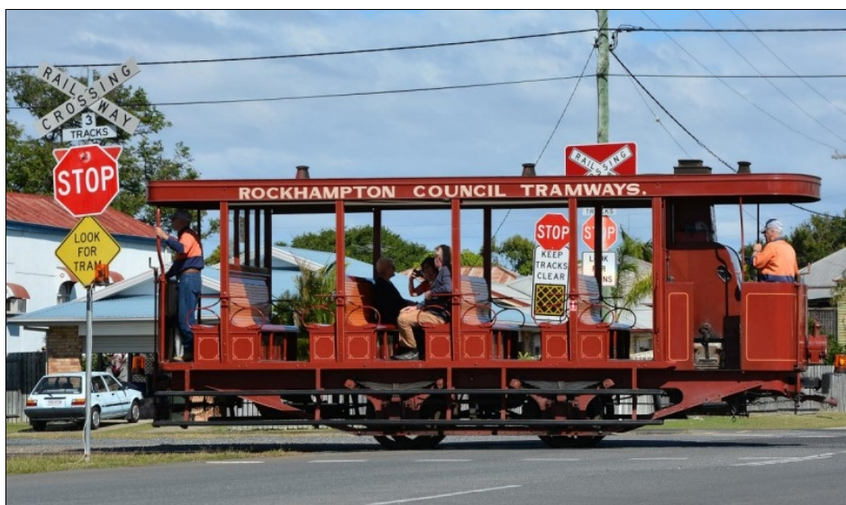
A restored Purrey Steam tram in Rockhampton, Qld. The driver is at left and a stoker at right, attending the boiler and steam engine at the rear of the tram. This restored tram is thought to be the only one surviving anywhere. Image by Mal Rowe in the Trams DownUnder website archive.
