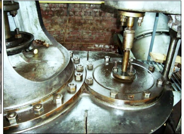
High pressure cylinders of the Duke & Orr pumping engine, with the top of the low pressure cylinders below them, and just projecting above the operating platform. Photographed through the glass wall, hence the shadowy reflections of metal grilles. Image: Owen Peake.
