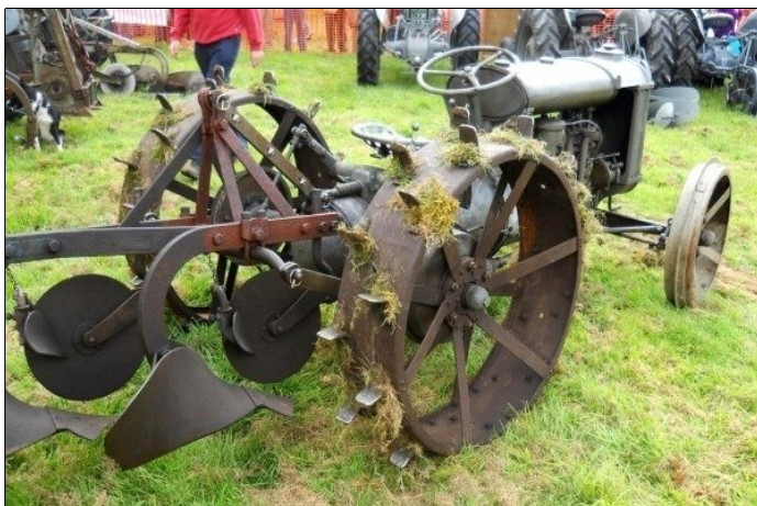
A 1936 steel-wheeled Ferguson-Brown tractor, with 3-point linkage holding a twin-furrow plough. Image: from a recent Fergie Field Day in the UK.
