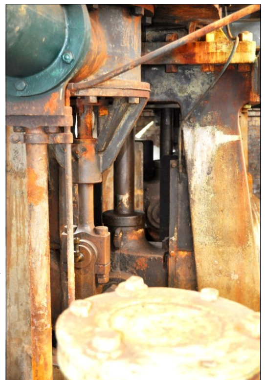
Main pump casing (foreground), the engine behind it, and the 2 nd pump casing just visible behind that – all before repainting. In the background is Paul Stephens, President of ISSSES, on a visit to Australia. Image: Owen Peake.
