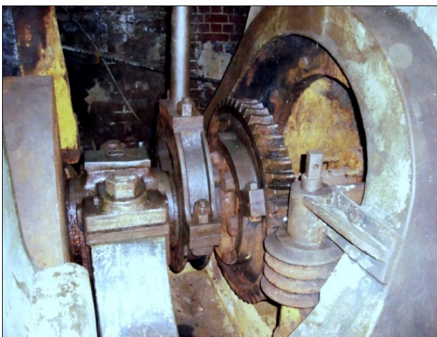
Engine crankshaft with main engine bearing (left), valve eccentric strap, turning gear and pump casing (right). Still much cleaning and polishing to be done. Image: Owen Peake.
