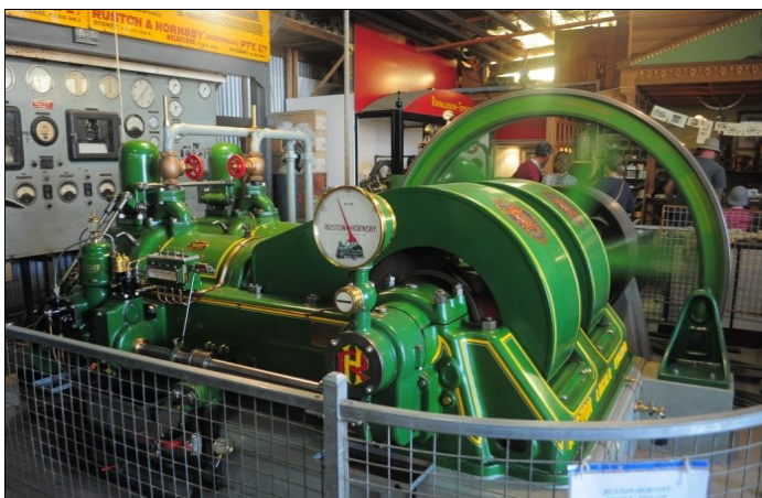
2 cylinder Ruston & Hornsby diesel engine c1930s in action. Note the whirring fly wheel, about 2m diameter. These engines were used for power generation, saw mill drives, pumping and in factories. Image: Owen Peake.
