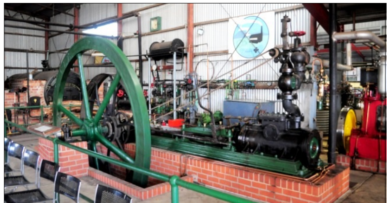
The Harrison steam mill engine, built in Ballarat c1880s. Image: Owen Peake.
